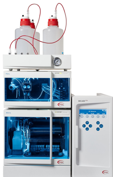
Figure 6: The ALEXYS analyzer for Amikacin EP, consisting of the ALEXYS Antibiotics base system - gradient, a dedicated flow cell, post-column kit and bottles. The base system consists of an AS6.1L autosampler, P6.1L pump quaternary LPG gradient pump, ET 210 Eluent tray for helium blanketing, and the DECADE Elite electrochemical detector. The post-column kit EP (not shown in figure) contains a P6.1L pump with solvent selection valve and dual channel degasser for post-column addition of NaOH. The system is delivered with DataApex™ Clarity™ Chromatography Data System (CDS) software. Optionally, control drivers are available to operate the system in Thermo Scientific™ Chromeleon™ CDS (version 7.2 SR 5 and up).
